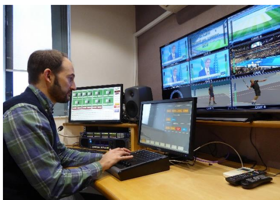
Figure 3 Voice Over booth with no fader controls required. Simplified operation can be managed by the presenters.
