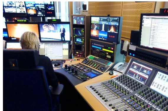
Figure 1. One operator taking control of both video and audio in automated live production
