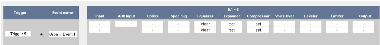
The Event named "Bypass Event1" may be triggered by "Trigger 5". It will turn the bypass **ON** for the function blocks: Expander, Compressor, and **OFF** for the Equalizer section.
