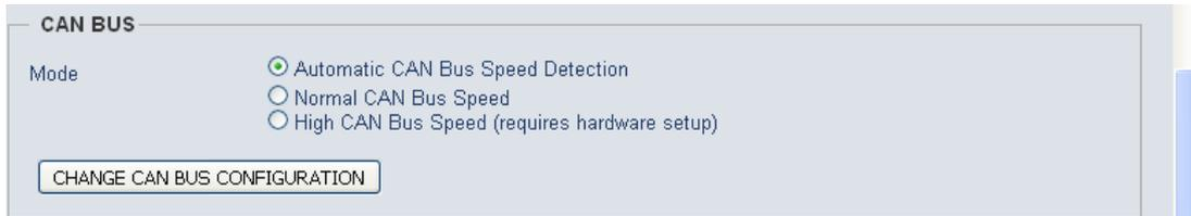
You can select between the two CAN bus speeds: **Normal** (125kBit/s) or **High** (1Mbit/s) and the **Automatic** detection of the installed modules.
