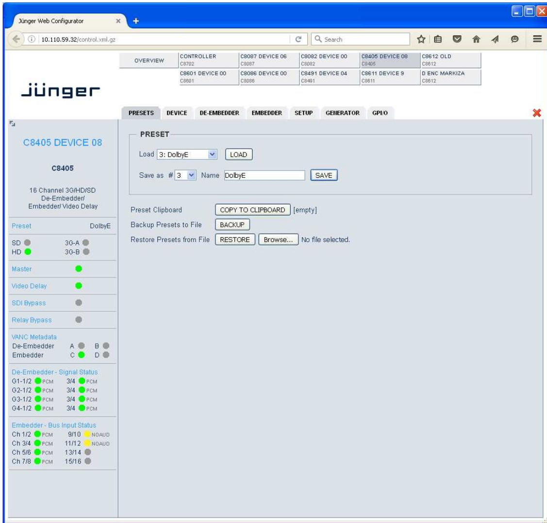
The **C8405** has **16 Presets**. These Presets are named **PRESET 01** to **PRESET 16** by default. The status window at the left hand side shows the name of the active preset. The word **“modified:”** will appear in line with the Preset name, if a preset parameter was changed by the operator.
