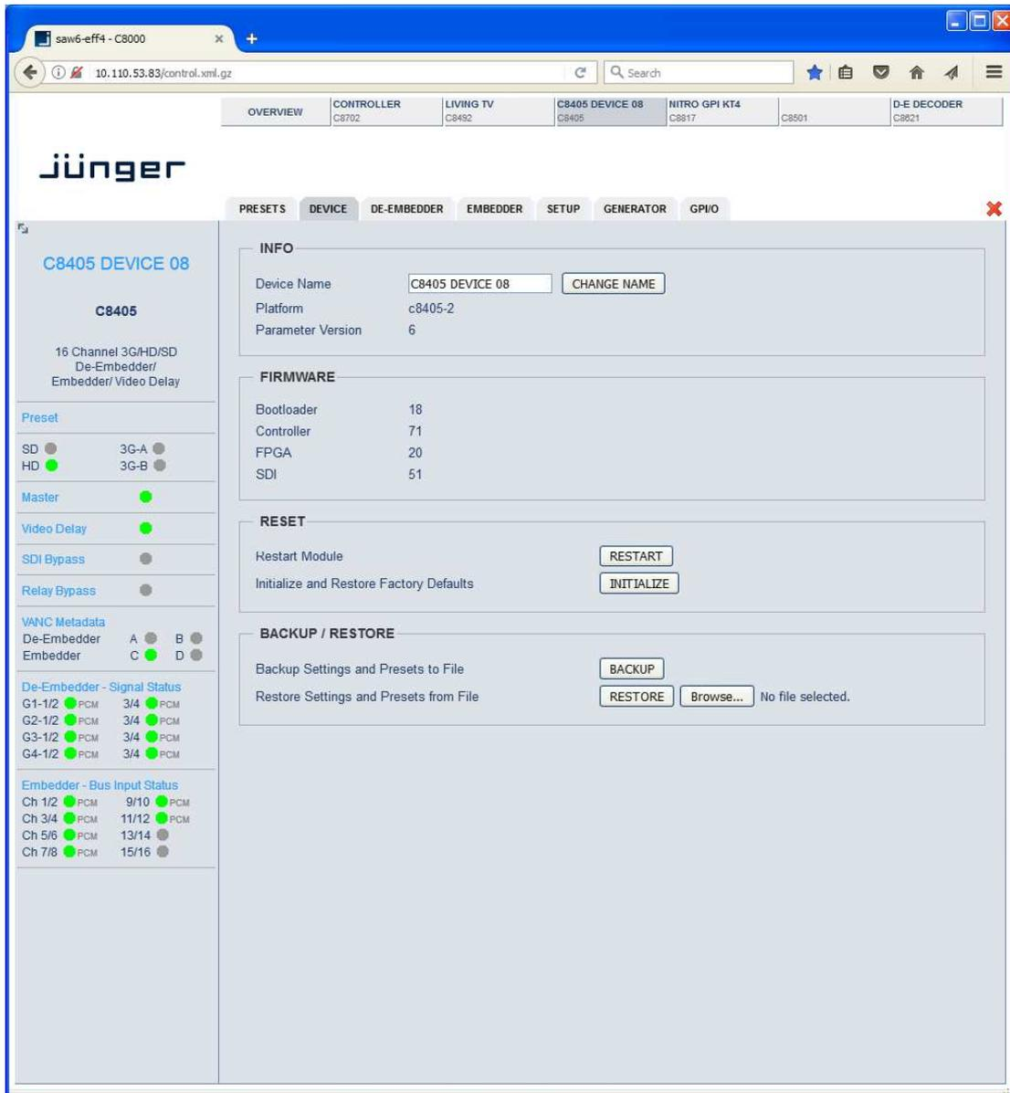
On the **DEVICE** page you can assign a **16 digit name** to the module, perform a warm start by pressing **<RESTART>** or initialize the module to factory default settings by pressing **<INITIALIZE>**.
