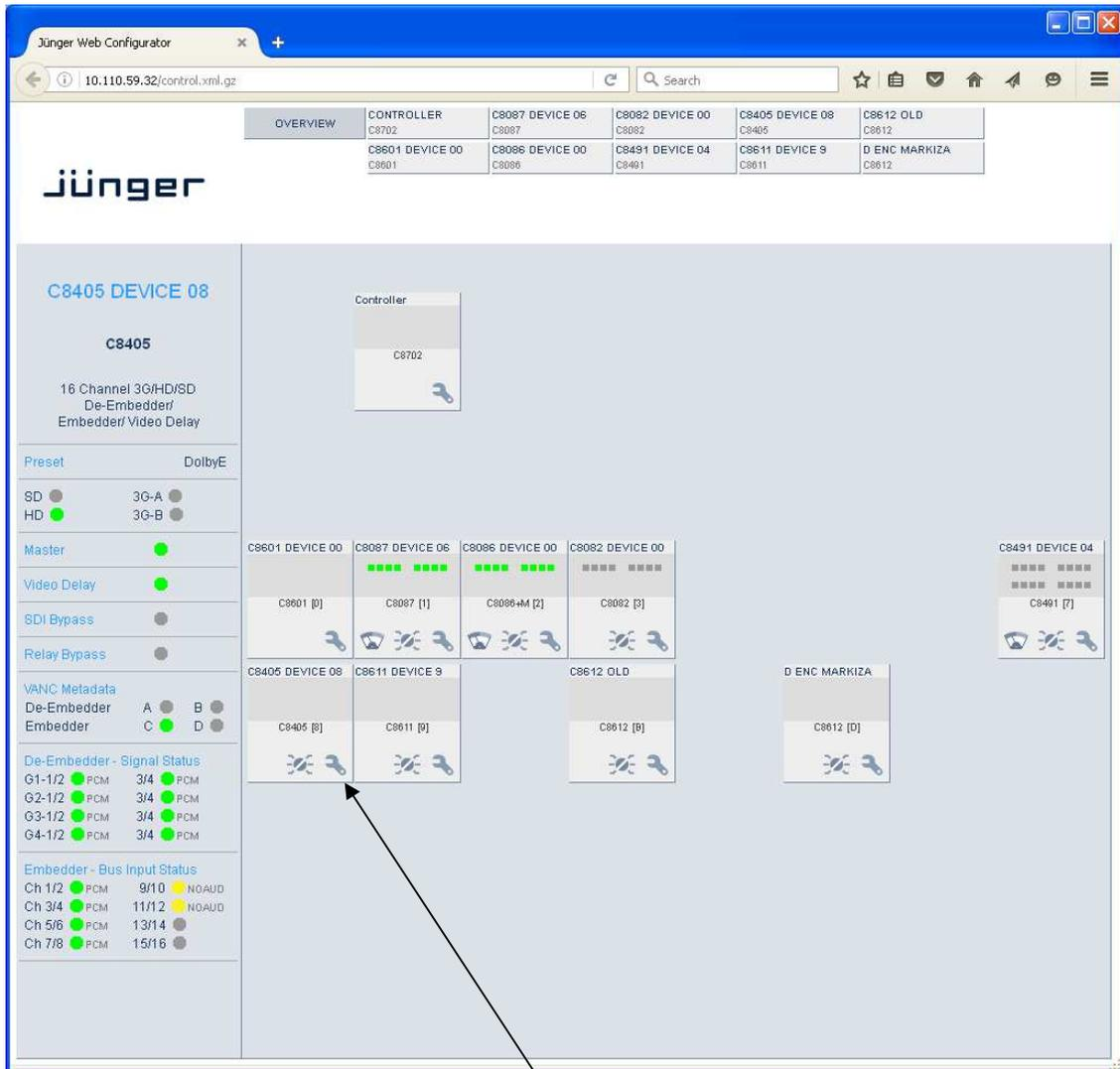
By simply clicking on the spanner tool symbol ● you will get the control pages of the **C8405** and the status window on the left side, which you will also see on mouse over. The entrance to the module setup is the **PRESET** page:
