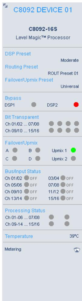
**C8092 DEVICE 01** - Given name of the module (may be changed on the DEVICE pane). It will be default set during initialization to module type amended by the word **DEVICE** and the CAN address **01** the module had at that moment.
